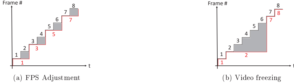
Fig. 11: The new metric, area loss, is designed to indicate the level of video freezing and the frame delay caused by insufficient bandwidth. The metric is less sensitive to the frame rate drops caused by the frame rate adjustment of systems.
